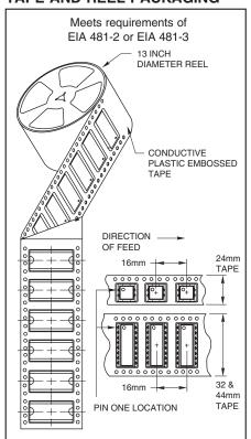
Each reel has a 15.750 inch (390 mm) minimum leader and a 6.30 inch (160 mm) minimum trailer.
