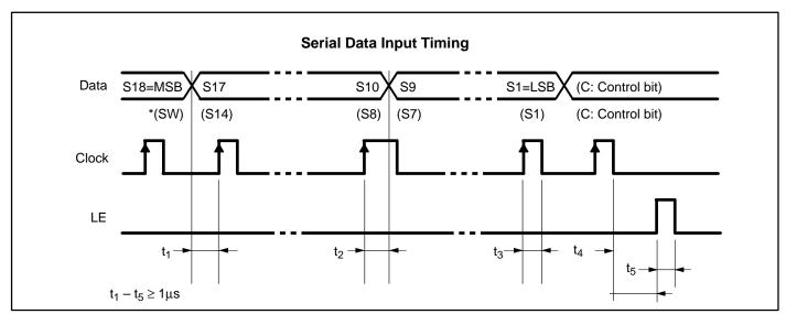
**NOTES:** Parenthesis data is used for setting divide ratio of programmable reference divider. On rising edge of clock shifts one bit of data in the shift register.
