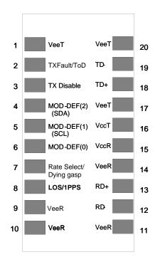
Pinout of Connector Block on Host equipment
