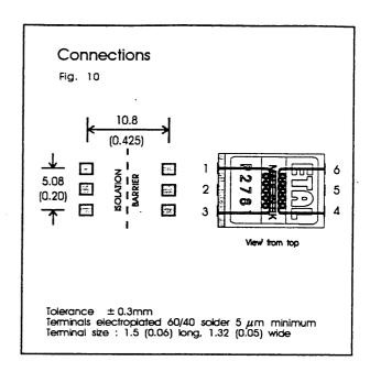
Dimensions shown are in millimetres (inches). Geometric centres of outline and pad grid coincide within a tolerance circle of 0.3mmØ. Windings may be used interchangeably as primary or secondary.
