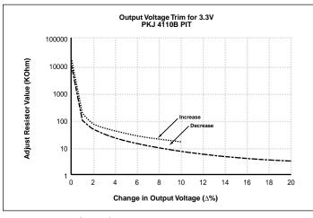
Decrease: Radj =  $\left(\frac{100}{\Delta \$} - 2\right) K\Omega$ Increase: Radj =  $\left[\frac{3.3 (100 + \Delta\%)}{1.225 \Delta\%} - \frac{(100 + 2\Delta\%)}{\Delta \$}\right] K\Omega$  These modules incorporate the same trim equation as used by some other major DC/DC converter suppliers. To decrease  $V_{\rm O}$  connect Radj from - SEN to Trim To increase  $V_{\rm O}$  connect Radj from + SEN to Trim
