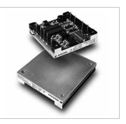
The PKJ 4000B series represents another one of Ericsson's "industry first" achievements in the continued development of our "Third Generation" of high-density, high-efficiency power modules. This module packs 48.2 W/in<sup>3</sup> at 92% efficiencies (3.3V @ 40A) in an industry standard half-brick package. These breakthrough features come from using the most advanced patented topology utilizing integrated magnetics and synchronous rectification on a low-resistivity multilayer PCB.
