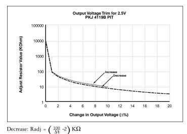
Increase: Radj =  $\begin{bmatrix} 2.5 (100 + \Delta\%) \\ 1.225\Delta\% \end{bmatrix} - \frac{(100 + 2\Delta\%)}{\Delta\%} K\Omega$
