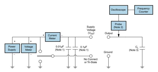
Note 1: An external 0.1µF low frequency tantalum bypass capacitor in parallel with a 0.01µF high frequency ceramic bypass capacitor close to the package ground and V<sub>DD</sub> pin is required.
