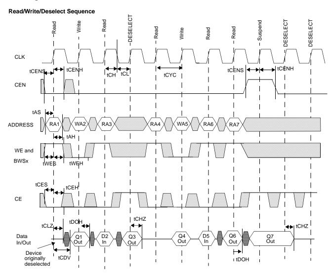
The combination of WE and BWSx (x = a, b, c, d) to define a Write cycle (see Write Cycle Description table). CE is the combination of CE1, CE2, and CE3. All chip selects need to be active in order to select the device. Any chip select can deselect the device. RAx stands for Read Address X, WA stands for Write Address X, Dx stands for Data-in X, Qx stands for Data-out X.
