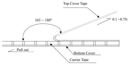
The peel speed shall be about 300 mm/minute
