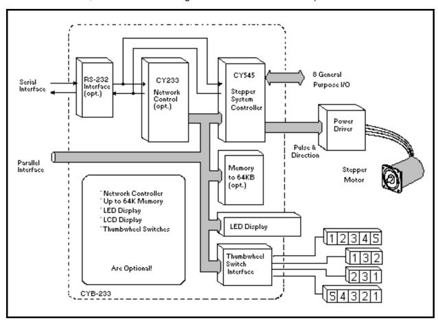
The CY545 can be commanded directly through its own serial port connection, or serially through the CY233 and the parallel CY545 interface. With this second option, it is possible to control multiple CY545s through one host serial port, as a network of motor controllers. The CY233 acts as the network communications controller, recognizing commands meant for the local CY545, while the CY545 runs the stepper motor as commanded by the host.
