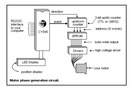
The data outputs from the PROM are then connected to the power driver circuit itself, generating the proper phase patterns for the motor. Note that such a design not only handles motors of various phases, but can also implement stepping schemes such as half-step or quadstep, as well as the standard full-step pattern.
