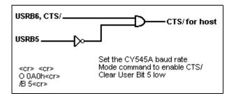
Finally, if MB6 is one, the CY545 uses the lower four bits of the mode byte value to select the serial baud rate. This allows a parallel command to set the serial rate to a desired value, without tying the I/O Request and Busy lines to a particular state, and allows a parallel command source to set up the CY545 for serial communications, such as showing messages on a serial display.
