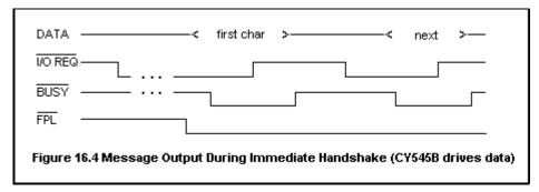
After the CY545B has issued the output message, and FPL is high again, the host may continue with the immediate command handshake, and the CY545B will now accept and execute the immediate command as shown in the second example waveform below. Here, the host does not drive the data bus for the first handshake, and thereby gives the CY545B the "0FFh" first command character prefix. This is followed by the normal first command character.
