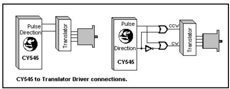
If the user opts for his own driver design, the PULSE and CCW lines may be used to drive a counter circuit, which counts up or down once for each pulse, based on the level of the CCW signal. The counter output then drives the address lines of a memory device, such as a PROM, EPROM, or EEPROM, with data outputs that generate the desired motor phase patterns as the counter address steps through the PROM locations. This design is shown here.
