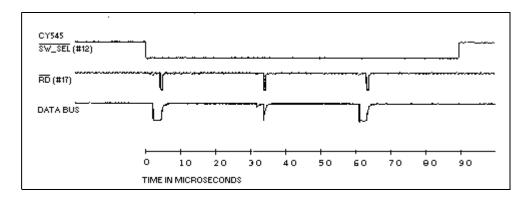
To read an entire parameter, the digit read process is repeated three, five, or eight times, depending on the size of the parameter. The CY545 starts by reading the most significant digit, then the next, until it finally reads the least significant digit. This is the same order that digits are read from a command with numeric arguments.
