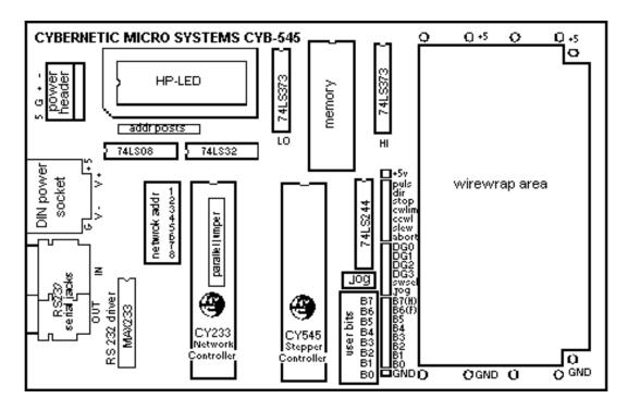
A Wirewrap area is provided for implementation of thumbwheel switches, driver circuits, or other custom circuitry. Based in the single height VME format (100mm x 160mm, approximately 4" x 6.3"), the board requires only +5v (@650mA). The RS232 level voltages are generated by the Max233 on the board.
