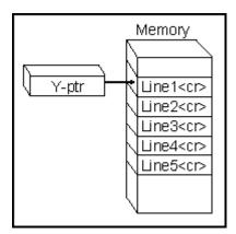
The memory display starts by showing the value of the memory address pointer, since the query will start at this address. This is followed by the number of lines specified by the count value. Each carriage return read from the memory counts as one line. This format operates in the ASCII command mode.
