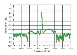
Figure 3: Band 25 Rx-Ant Insertion Loss
