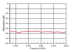
Figure 13: Band 25 Tx-Ant Attenuation in Bluetooth/ISM Bands
