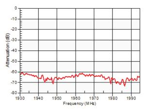
Figure 37: Band 66 Tx-Ant Attenuation at Tx Second Harmonic
