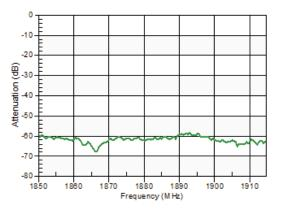
Figure 50: Cross-Band Isolation, Band 66 Tx to Band 25 Rx in Band 25 Rx, 1930-1995 MHz
