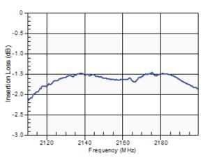
Figure 27: Band 66 Ant-Rx Insertion Loss
