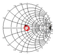
Figure 47: Band 66 Impedance, Ant (black) and Rx (blue) Ports, 2110–2200 MHz
