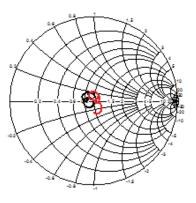
Figure 25: Band 25 Impedance, Ant (black) and Rx (blue) Ports, 1930–1995 MHz
