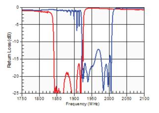
Figure 7: Band 25 Antenna Port Return Loss
