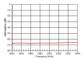
Figure 38: Band 66 Tx-Ant Attenuation at Tx Third Harmonic
