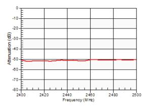
Figure 14: Band 25 Tx-Ant Attenuation at Tx Second Harmonic
