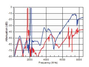
Figure 34: Band 66 Tx-Ant Attenuation in GNSS Bands
