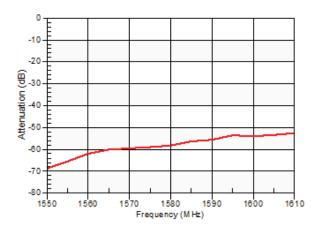
Figure 36: Band 66 Tx-Ant and Ant-Rx Attenuation in Bluetooth Band
