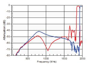
Figure 11: Band 25 Tx-Ant Attenuation in Band 66 Rx, 2110–2200 MHz
