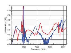
Figure 10: Band 25 Tx-Ant Attenuation in GNSS Bands
