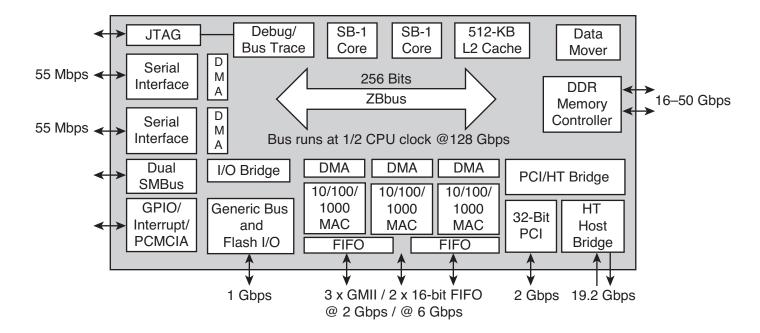
Broadcom's first SiByte<sup>TM</sup> processor, the **BCM1250**, is a state-of-the-art multiprocessor solution targeted at the fast-growing networking and communications markets.
