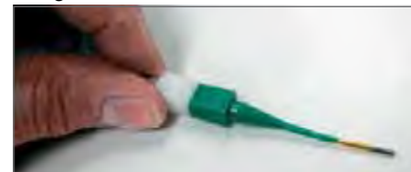
Plastic tool with contact in proper position.
