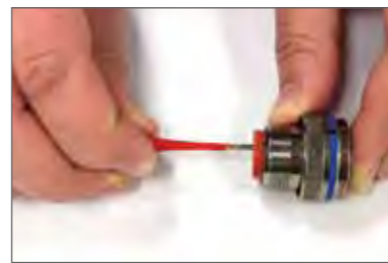
Plastic tool with contact in proper position.
