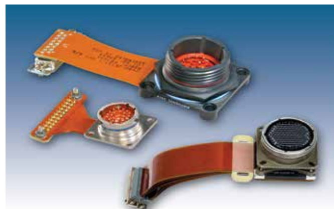
Flex Termination for Attachment to PC Boards
