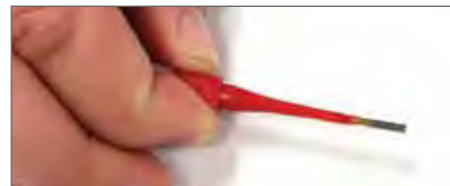
Plastic tool with contact in proper position.
