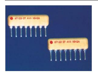
SIP-style, MLC ceramic capacitor arrays are Single-In-Line, conformally coated packages. These capacitor networks incorporate multiple capacitors into a single substrate and, therefore, offer excellent TC tracking. The utilization of SIP capacitor arrays minimizes board real estate and reduces component count in the assembly. Various circuit configurations and capacitance/voltage values are available.
