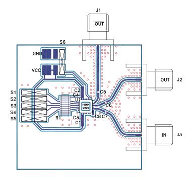
The circuit board used in the application should use RF circuit design techniques. Signal lines should have 50 Ohm impedance while the package ground leads and backside ground slug should be connected directly to the ground plane similar to that shown. A sufficient number of via holes should be used to connect the top and bottom ground planes. The evaluation circuit board shown is available from Hittite upon request.
