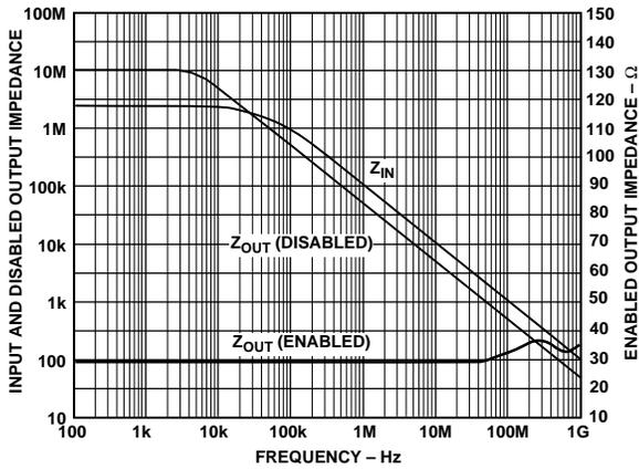
Figure 16. Output & Input Impedance vs. Frequency
