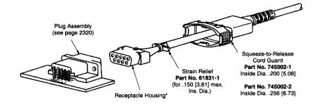
\*Squeeze-to-Release Cord Guards also can be used on plug housings (shown above).
