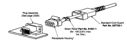
\*Standard Cord Guards also can be used on plug housings (shown above).
