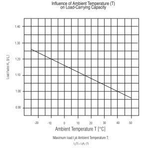
The 1489-A circuit breaker can function over a wide temperature range (-30°....+60° C). Operation in ambient temperatures below 0° C is based on a non condensing atmosphere (no ice). Use the graph above or contact your local Rockwell Automation sales office or Allen-Bradley distributor to determine the correction factor based upon ambient temperature.
