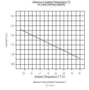
The 1489-D circuit breaker can function over a wide temperature range (-30°....+60°C). Operation in ambient temperatures below 0°C is based on a non condensing atmosphere (no ice). Use the graph above or contact your local Rockwell Automation sales office or Allen-Bradley distributor to determine the correction factor based upon ambient temperature.
