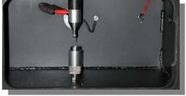
The Model 949 Test Target is a current transducer with  $50\Omega$  impedance and frequency response to 2 GHz that is used to measure all ESD output waveforms. It has a transfer ratio of 1 Volt/amp. A 3' (91cm) RG58 cable is included. The Model 949 is designed in accordance with IEC 61000-4-2
