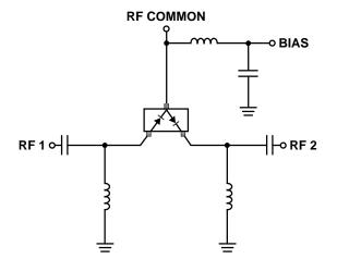
Figure 14. Switch Using Both Positive and Negative Bias Current.
