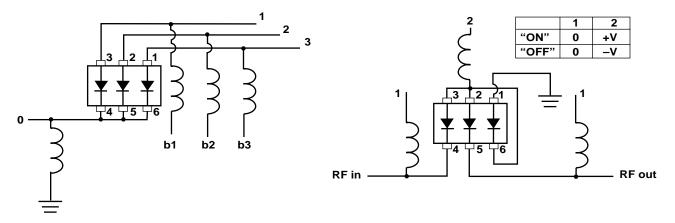
Figure 6. HSMP-389L used in a SP3T Switch.
