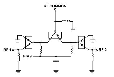
Figure 15. Very High Isolation SPDT Switch, Dual Bias.
