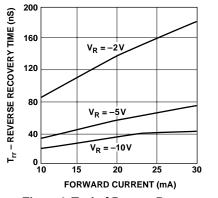
Figure 4. Typical Reverse Recovery Time vs. Reverse Voltage.
