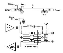
Figure 10. HSMP-389U Series/Shunt Pair used in a 900 MHz Transmit/Receive Switch.
