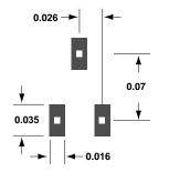
Figure 23. PCB Pad Layout, SOT-323. (dimensions in inches).
