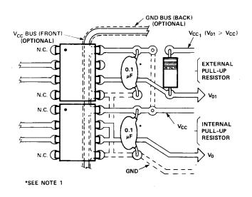
Figure 19. Recommended Printed Circuit Board Layout.
