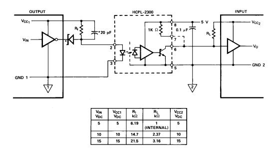
\*SCHOTTKY DIODE (HP 5082-2800, OR EQUIVALENT) AND 20 pF CAPACITOR ARE NOT REQUIRED FOR UNITS WITH OPEN COLLECTOR OUTPUT.
