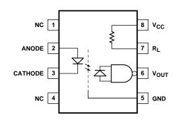
A 0.1 pF bypass capacitor must be connected between pins 5 and 8.
