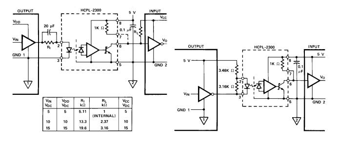
Figure 13. Active CMOS Series Drive Circuit.
