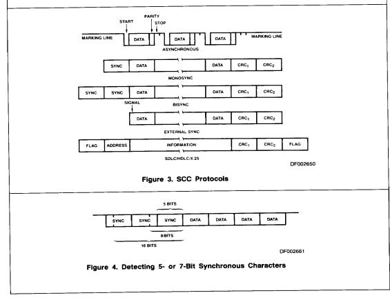
CRC checking for Synchronous byte-oriented modes is delayed by one character time so that the CPU may disable CRC checking on specific characters. This permits the implementation of protocols, such as IBM Bisync.
