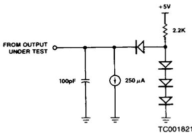
Open Drain Test Load
