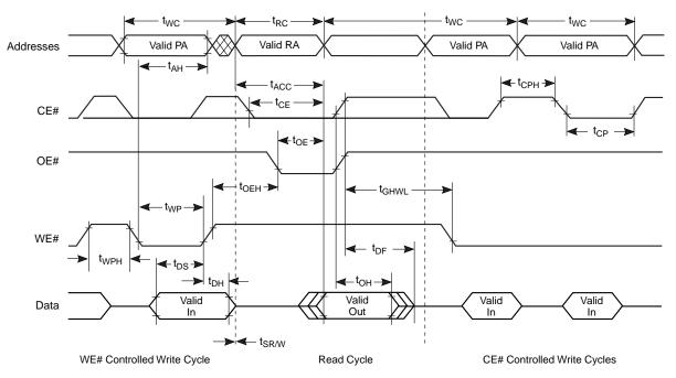
Figure 19. Back-to-Back Read/Write Cycle Timings
