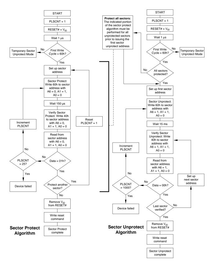
Figure 2. In-System Sector Protect/Unprotect Algorithms
