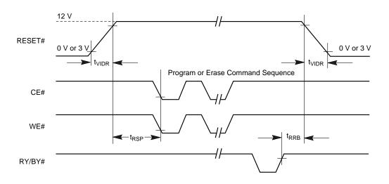
Figure 23. Temporary Sector Unprotect Timing Diagram
