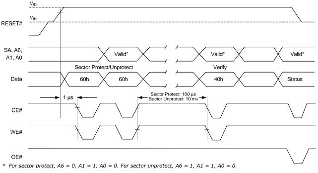
Figure 24. Sector Protect/Unprotect Timing Diagram
