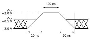
Figure 8. Maximum Positive Overshoot Waveform
