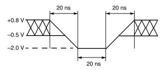
Figure 7. Maximum Negative Overshoot Waveform
