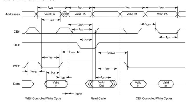
Figure 20. Back-to-back Read/Write Cycle Timings
