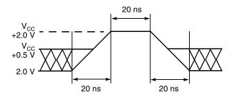
Figure 8. Maximum Positive Overshoot Waveform
