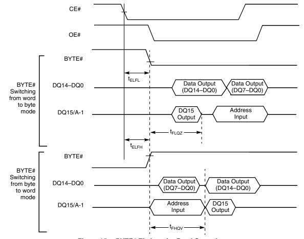
Figure 15. BYTE# Timings for Read Operations
