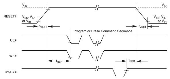
Figure 24. Temporary Sector Unprotect Timing Diagram
