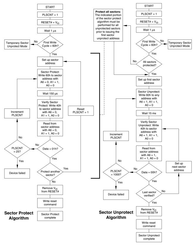
Figure 2. In-System Sector Protection/ Sector Unprotection Algorithms
