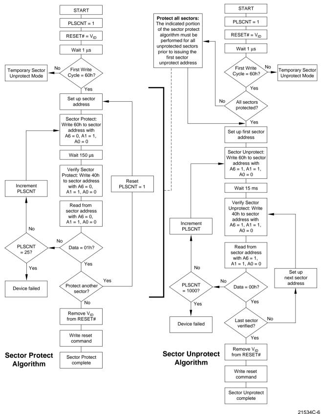
Figure 2. In-System Sector Protect/Unprotect Algorithms
