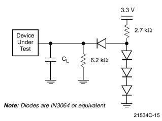
Figure 11. Test Setup
