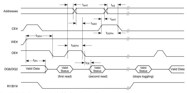
**Note:** VA = Valid address; not required for DQ6. Illustration shows first two status cycle after command sequence, last status read cycle, and array data read cycle
