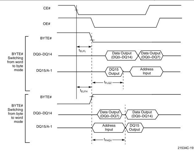
Figure 15. BYTE# Timings for Read Operations
