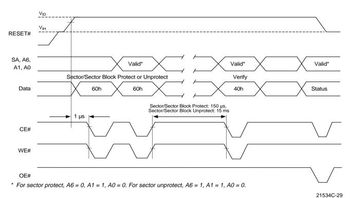
Figure 25. Sector/Sector Block Protect and Unprotect Timing Diagram
