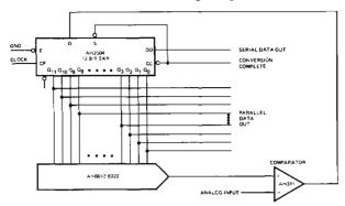
This shows how the Am2502/3/4 registers are used with a Digital-to-Analog converter and a comparator to form a very high-speed continuous conversion Analog-to-Digital converter. Conversion time is limited mainly by the speed of the D/A converter and comparator with typical conversion rates of 100,000 conversions per second.
