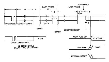
\* The configuration data consists of a composite 40-bit preamble/length count, followed by one or more concatenated LCA programs, separated by 4-bit postambles. An additional final postamble bit is added for each slave device and the result rounded up to a byte boundary. The length count is two less than the number of resulting bits. Timing of the assertion of DONE and termination of the INTERNAL RESET may each be programmed to occur one cycle before or after the I/O outputs become active.
