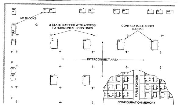
Figure 1. Logic Cell Array Structure. It consists of a perimeter of programmable I/O blocks, a core of configurable logic blocks and their interconnect resources.
