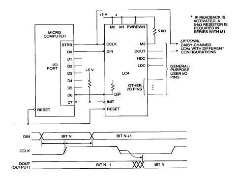
Figure 24. Slave Mode. Bit-serial configuration data are read at rising edge of the CCLK.
