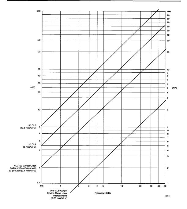
Figure 31. LCA Device Power Consumption by Element. Total chip power is the sum of Vcc•lcco plus effective internal and external values of frequency dependent capacitive charging currents and duty factor dependent resistive loads.
