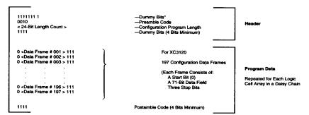
\*The LCA Device Require Four Dummy Bits Min; XACT Software Generates Eight Dummy Bits
