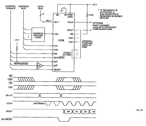
Figure 23. Peripheral Mode. Configuration data are loaded using a byte-wide data bus from a microprocessor.
