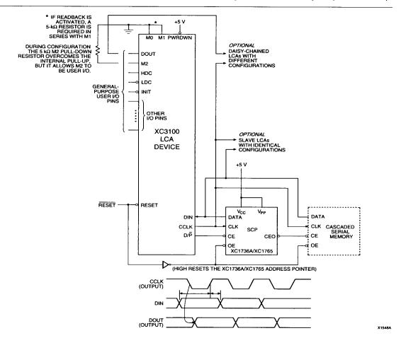
Figure 21. Master Serial Mode. The one-time-programmable XC1736A/XC1765 Serial Configuration PROM supports automatic loading of configuration programs up to 36K/64K bits. Multiple devices can be cascaded to support additional LCA devices. An early D/P inhibits the PROM data output a CCLK cycle before the LCA I/Os become active.
