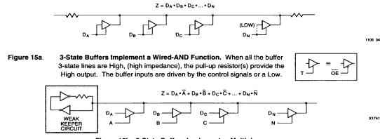
Figure 15b. 3-State Buffers Implement a Multiplexer. The selection is accomplished by the buffer 3-state signal.
