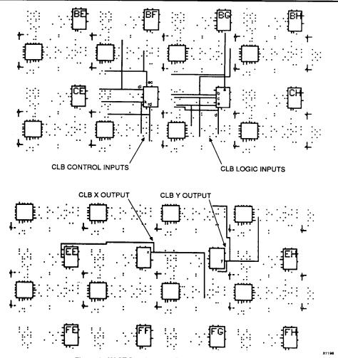
Figure 8. XACT Development System Locations of interconnect access, CLB control inputs, logic inputs and outputs. The dot pattern represents the available programmable interconnection points (PIPs).
