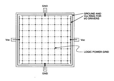
Figure 30. LCA Device Power Distribution.
