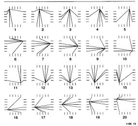
Figure 10. Switch Matrix Interconnection Options for Each Pin. Switch matrices on the edges are different.
