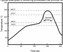
Fig. 2 Infrared soldering profile
