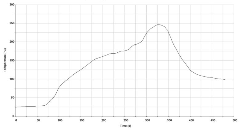
Figure 8: Typical Lead-free Reflow Solder Profile
