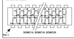
TTL dual-line terminator; pulse squaring, 12, 14, or 18 pairs of resistors (R<sub>1</sub> resistors are common to leads 14, 16, or 20)
