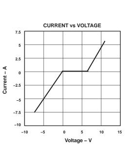
NOTE A: Typical current versus voltage curve was derived using the IEC 1.2/50-µs surge waveform.
