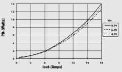
Note 1: All data listed in the above graphs bas been developed from actual products tested at 25°C. This data is considered typical data for the ISR. Note 2: SOA curves represent operating conditions at which internal components are at or below manufacturer's maximum rated operating temperatures.
