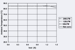
**Note A:** Characteristic data has been developed from actual products tested at 25°C. This data is considered typical data for the ISR. **Note B:** SOA curves represent operating conditions at which internal components are at or below manufacturer's maximum rated operating temperatures.
