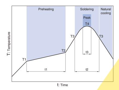
Soldering Preheating Peak Temp. Time Temp. Time Temp. Time T2 Т3 150°C 180°C 90 to 120s 230°C 10s max 40s 255°C
