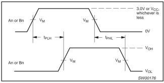
Waveform 2. Propagation Delay, Transparent Mode
