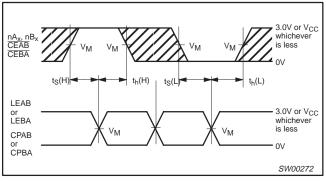
Waveform 4. Data Setup and Hold Times
