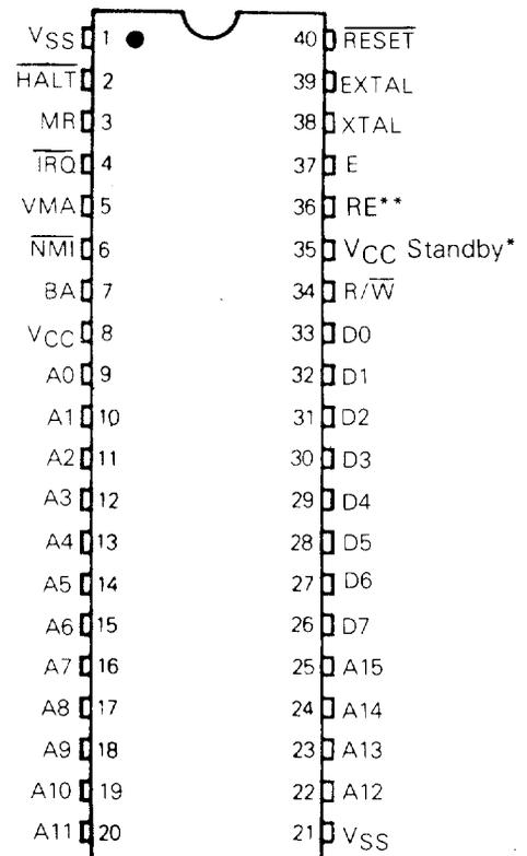
\* Pin 35 must be tied to 5 V on the MC6802NS
