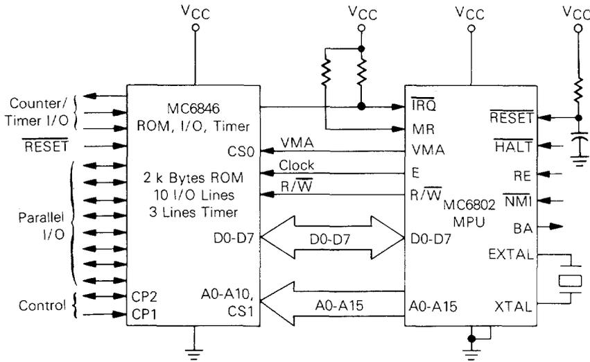
This block diagram shows a typical cost effective microcomputer. The MPU is the center of the microcomputer system and is shown in a minimum system interfacing with a ROM combination chip. It is not intended that this system be limited to this function but that it be expandable with other parts in the M6800 Microcomputer family.
