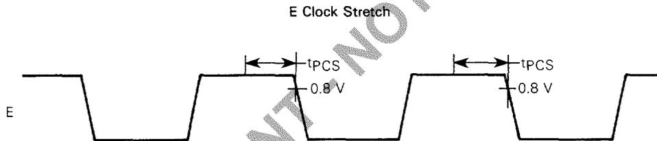
The E clock will be stretched at end of E high of the cycle during which MR negative meets the  $t_{PCS}$  setup time. The  $t_{PCS}$  setup time is referenced to the fall of E. If the  $t_{PCS}$  setup time is not met, E will be stretched at the end of the next E-high  $\frac{1}{2}$  cycle. E will be stretched in integral multiples of  $\frac{1}{2}$  cycles.
