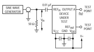
Figure 8. Test Circuit — Reference Mode
