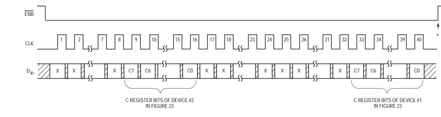
\*At this point, the new bytes are transferred to the C registers of both devices and stored. No other registers are affected.
