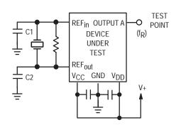
Figure 9. Test Circuit — Crystal Mode
