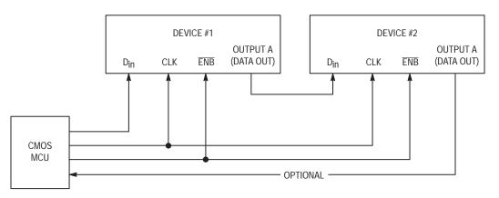
NOTE: See related Figures 24 through 26; these bit streams apply to the MC145190, MC145191, MC145200, and MC145201.
