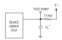
\*Includes all probe and fixture capacitance.
