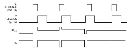
NOTE: The PD output state is equal to either V<sub>DD</sub> or V<sub>SS</sub> when active. When not active, the output is high impedance and the voltage at that pin is determined by the low–pass filter capacitor.
