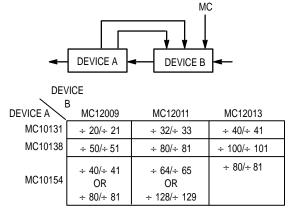
NOTE: MC12009, MC12011, and MC12013 are pin equivalent. MC12015, MC12016, and MC12017 are pin equivalent.
