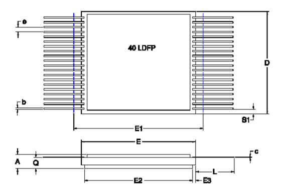
40 PIN RAD-TOLERANT FLAT PACKAGE DIMENSIONS
