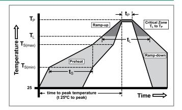
Wave Soldering Parameters
