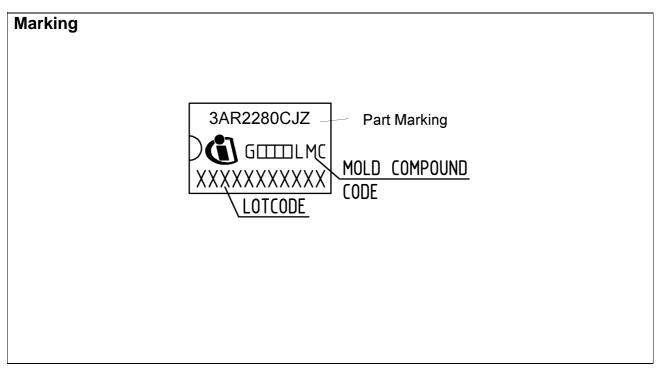
Figure 41 Marking for ICE3AR2280CJZ
