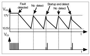
Figure 26 Odd skip auto restart waveform
