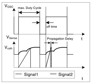
Figure 21 Dynamic Voltage Threshold V<sub>csth</sub>
