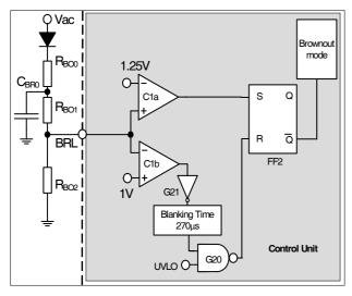
Figure 30 Brownout detection circuit
