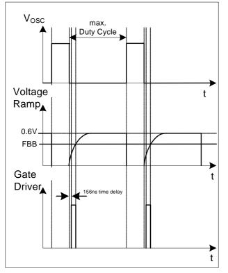
7). It allows the duty cycle to be reduced continuously till 0% by decreasing  $V_{\text{FBB}}$  below that threshold.
