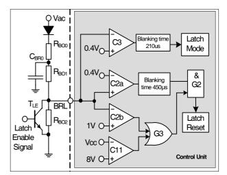
Figure 32 Latch and fast AC reset
