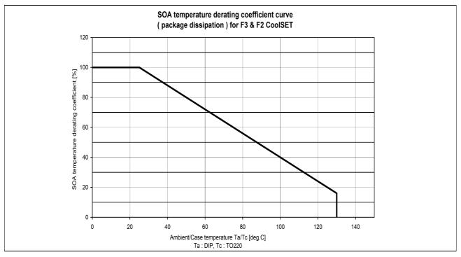
Figure 35 SOA temperature derating coefficient curve
