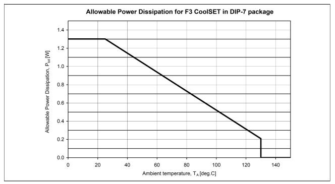
Figure 36 Power dissipation;  $P_{tot}=f(T_a)$
