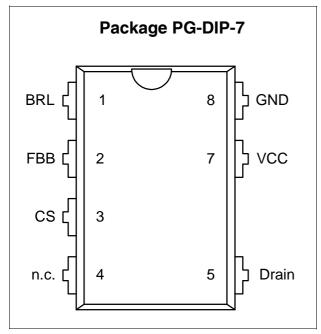
Figure 1 Pin Configuration PG-DIP-7 (top view)
