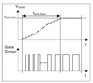
Figure 13 Gate drive signal under Soft-Start Phase
