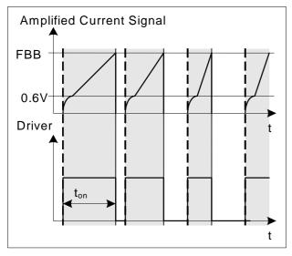
Figure 5 Pulse Width Modulation
