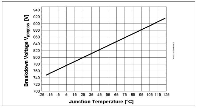
Figure 37 Drain-source breakdown voltage;  $V_{BR(DSS)}=f(T_i)$ ,  $I_D=0.25mA$
