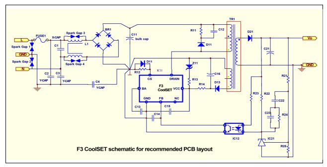
Figure 42 Schematic for recommended PCB layout
