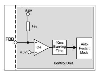
Figure 29 Over load and open loop protection
