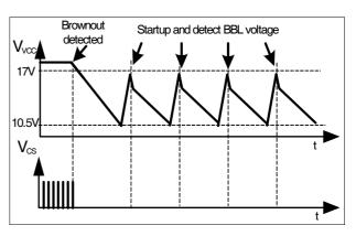
Figure 31 Brownout mode waveform
