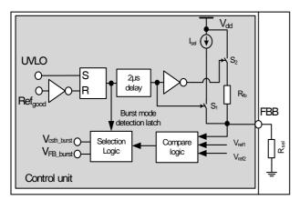
Figure 24 Burst mode detect and adjust
