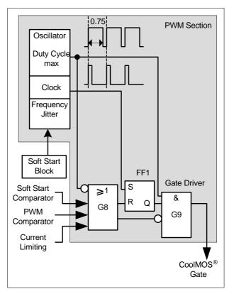
Figure 15 PWM Section Block
