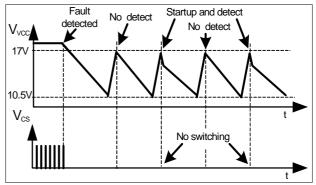
Figure 27 non switch auto restart waveform
