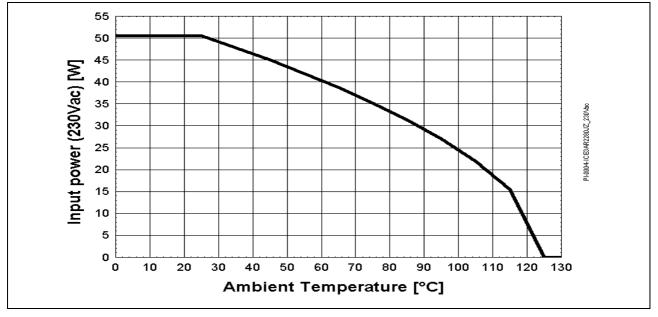
Figure 39 Input power curve Vin=230Vac+/-15%;  $P_{in}=f(T_a)$
