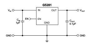
Note: Recommend connecting the Thermal Pad to the GND for excellent power dissipation.
