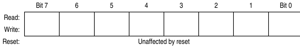
Figure 3-3. Index Register (X)
