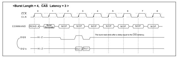
The Burst Terminate command is a mandatory feature for DDR SDRAMs. The following functionality is required.
