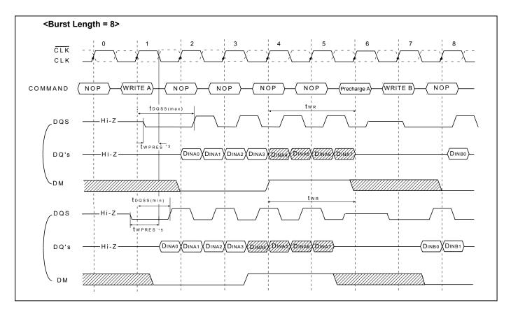
Precharge timing for Write operations in DRAMs requires enough time to allow "write recovery" which is the time required by a DRAM core to properly store a full "0" or "1" level before a Precharge operation. For DDR SDRAM, a timing parameter,  $t_{WR}$ , is used to indicate the required of time between the last valid write operation and a Precharge command to the same bank.
