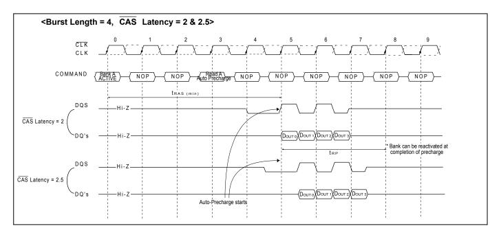
When the Read with Auto Precharge command is issued, new command can be asserted at 4, 5 and 6 respectively as follow.
