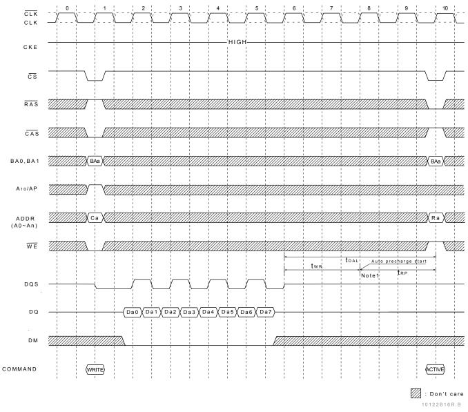
Note: 1. The row active command of the precharge bank can be issued after t<sub>RP</sub> from this point. The new read/write command of another activated bank can be issued from this point. At burst read/write with auto precharge, CAS interrupt of the same/another bank is illegal.
