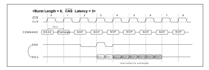
When a burst Read command is issued to a DDR SDRAM, a Precharge command may be issued to the same bank before the Read burst is complete. The following functionality determines when a Precharge command may be given during a Read burst and when a new Bank Activate command may be issued to the same bank.
