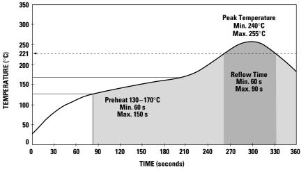
Figure 12. Surface Mount Assembly Temperature Profile.
