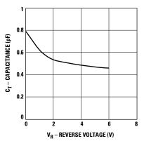
Figure 3. Total Capacitance vs. Reverse Voltage.
