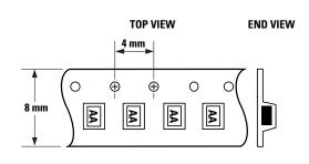
Note: "AA" represents package marking code. Package marking is right side up with carrier tape perforations at top. Conforms to Electronic Industries RS-481, "Taping of Surface Mounted Components for Automated Placement." Standard quantity is 3,000 devices per reel.
