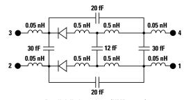
Parallel diode package (HMPx-x8x5)
