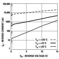
Figure 2. Reverse Current vs. Reverse Voltage at Temperatures.
