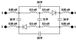
Anti-parallel diode package (HMPx-x8x2)
