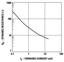
Figure 4. Dynamic Resistance vs. Forward Current.
