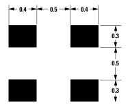
Figure 10. PCB Pad Layout, MiniPak (dimensions in mm).
