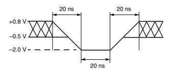
Figure 6. Maximum Negative Overshoot Waveform
