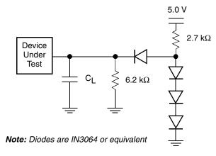
Figure 8. Test Setup
